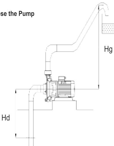
Hm(mSS) :Total Manometric Height (mSS)
