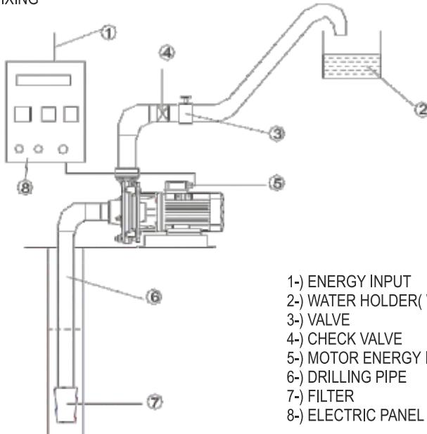
Before fitting, consider close point to fix the pump, measures taken to prevent the pump from outside effects, a dry point selection, proper selection of pump, close to energy line.
